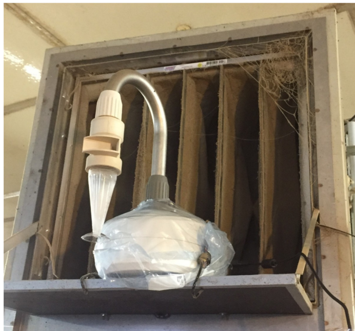
Fig 4. Position of the Coriolis ® \mu Air Sampler in front of the UVC module. The picture shows the Coriolis ® \mu Air Sampler operating on a mounted board in front of the pocket filter for measurements in close proximity to the UVC module.
